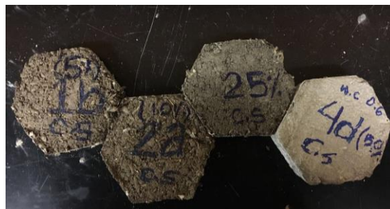
Figure 1: Prototypes made of Cotton stalk-cement
