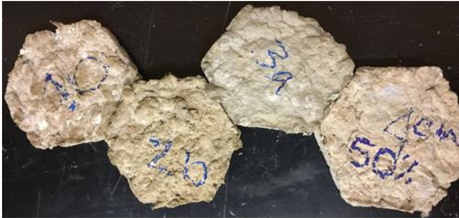
Figure 3: Cement as Binder: mold formation was observed
